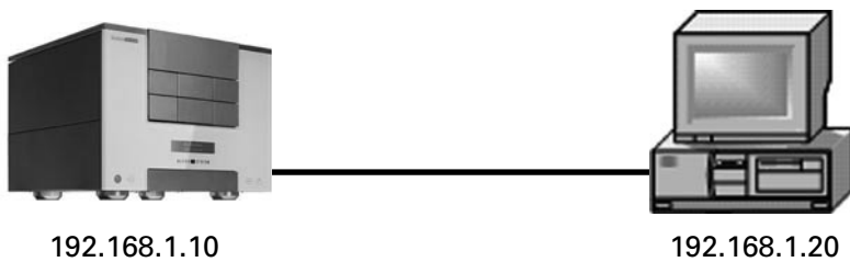
Direct connection between a PC and a Casablanca (via a crossover Ethernet cable)
