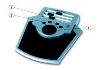
The Twister is equipped with three slider controls, which allow you to directly adjust video and audio settings. It also has four buttons that are responsible for different functions in various screens.
