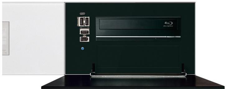
Open the large front panel on the right to get to the front connections and the optical drive(s) of the Karat / Topaz. Open the panel by pulling the glass at the top right corner of the device towards yourself. To do this, a slight resistance must be overcome. Since the panel is buffered, it will then come down automatically.
