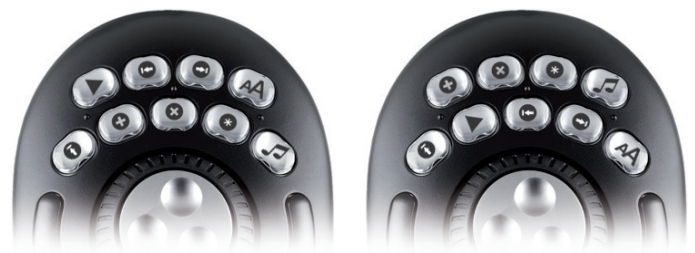
Assignments 1 and 2, with the corresponding symbol assignments for the buttons of the Shuttle TT
