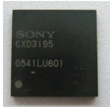
Figure 1: MPEG-2 HD codec LSI (13 mm per side)
