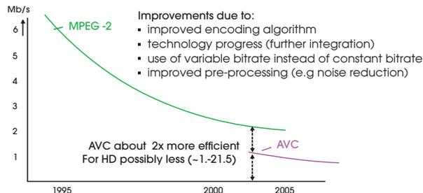
**Figure 3:** Improvements in compression efficiency of MPEG-2
